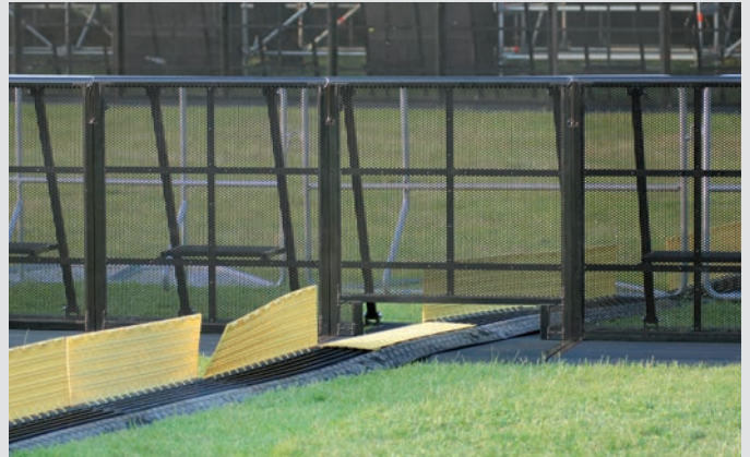
Specialized barricade to accommodate cables and wiring
